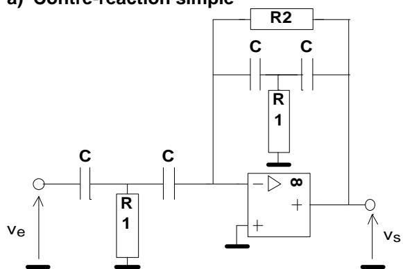
$$\omega_0 = \frac{1}{C\sqrt{R_1 \cdot R_2}} \quad C \text{ arbitraire}$$
