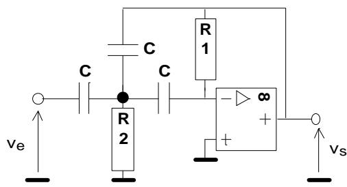
$$\omega_0 = \frac{1}{C\sqrt{R_1 \cdot R_2}} \quad C \text{ arbitraire}$$
