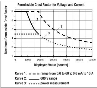
Above figure: Influence of Crest Factor on Display Range Additional error caused by the signal's crest factor:
