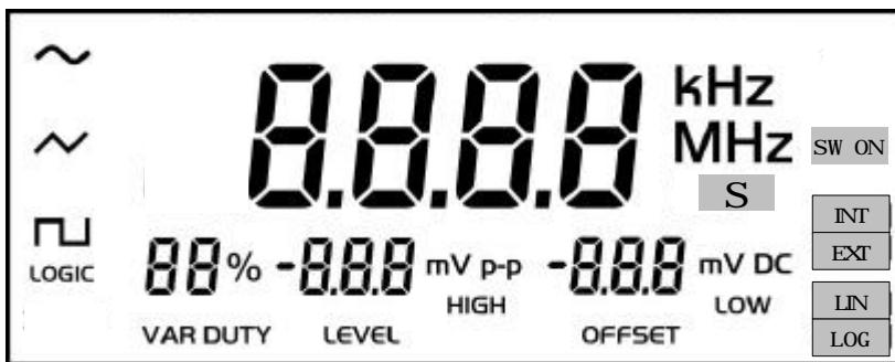
In this mode, specific symbols (grey in the view of the LCD above) are used in addition to the symbols of the function generator :
