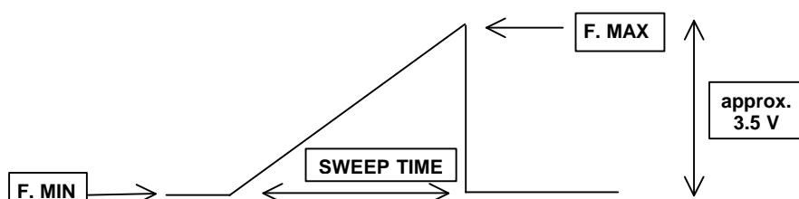
*Note 1: In internal SWEEP mode, the display indicates alternatively the low frequency "F. MIN" and high frequency "F. MAX".*
