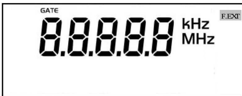
In this mode, the specific symbol (greyed in the LCD view) is used in addition to "88888", "GATE", "kHz", "MHz" described in the previous paragraphs.
