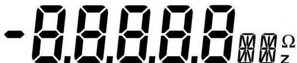
The 2 displays / 14 segments allow you to display a whole list of electric or physical magnitude measurement units.
