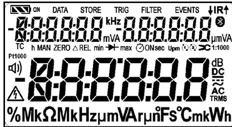
Transreflective LCD panel (65 x 36 mm) with display of up to 3 measured values, unit of measure, type of current and various special functions.
