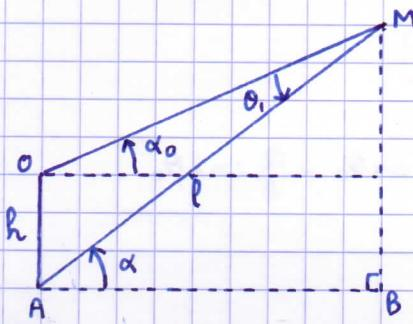
$$\text{On a: } \cos \alpha = \frac{AB}{l} \quad \text{et} \quad \cos \alpha_0 = \frac{AB}{OM}$$
