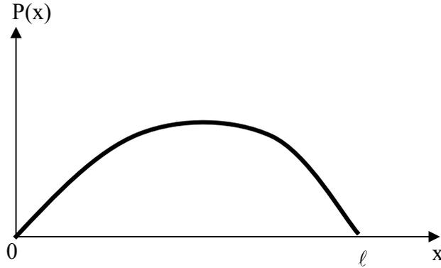
10-  $\boxed{F_y = \iint_{\text{plaque}} P(x) dx dz = L \int_0^{\ell} P(x) dx}$      et      $\boxed{F_x = \iint_{\text{plaque}} -\eta \frac{\partial v_x}{\partial y}(x,0) dx dz = L \int_0^{\ell} -\eta \frac{\partial v_x}{\partial y}(x,0) dx}$
