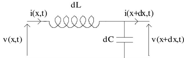
**Loi des mailles :**  $v(x,t) = dL \frac{\partial i}{\partial t}(x,t) + v(x+dx,t) \Rightarrow 0 = \Lambda dx \frac{\partial i}{\partial t}(x,t) + v(x+dx,t) - v(x,t)$
