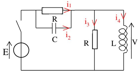
$$\text{On pose : } \omega_0 = \frac{1}{\sqrt{LC}} \text{ et } \frac{\omega_0}{Q} = \frac{2}{RC} \quad \text{Donc : } \boxed{\frac{d^2V}{dt^2} + \frac{\omega_0}{Q} \frac{dV}{dt} + \omega_0^2 V = 0}$$
