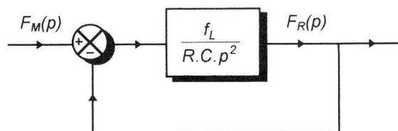
2.9  $T_{BO}(p) = \frac{f_L}{RCp^2}$        $T_{BO}(j\omega) = \frac{-f_L}{RC\omega^2}$
